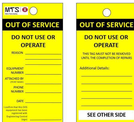
Figure 3 Out of service tag
