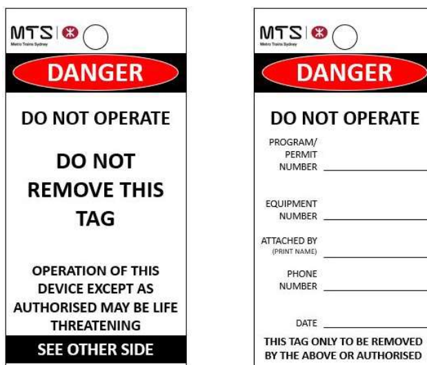
Figure 1 Danger - Do not operate tag
